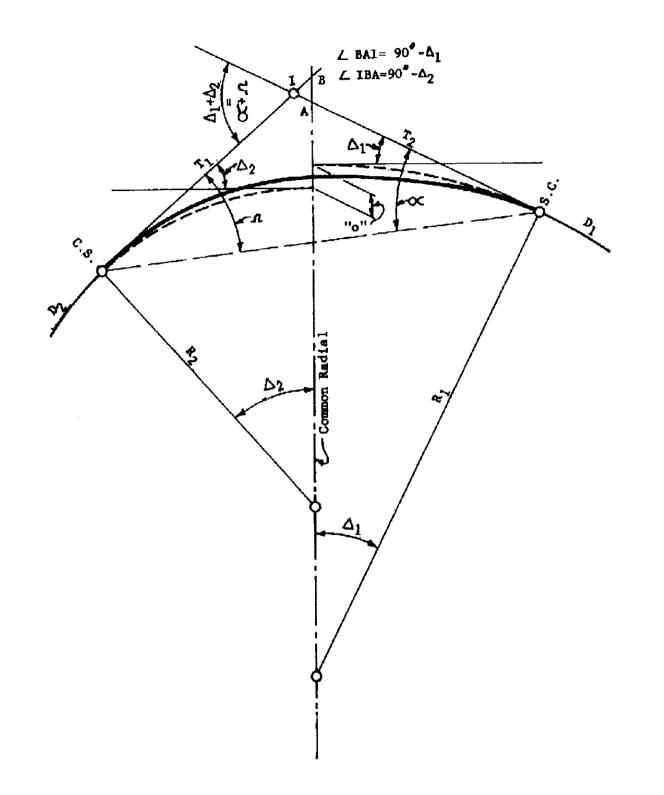
Intermediate Spiral Transition is basically the same as Partial Transition Spiral illustrated by Drwg. No D-55.20.
